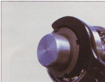
**E** Use a hook wrench to tighten the concave nut with a rated torque.
