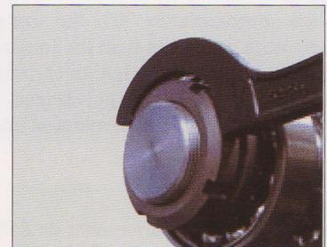
Tighten the concave nut with the wrench about 1 turn. The assembly can be inverted just in a case with the same results.
