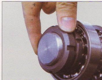
Screw the concave nut onto the shaft until its machined recess contacts the convex nut manually.
